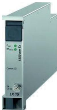
The WISI OPTOPUS LX 15 S 40x0 Transmitter series is part of WISI's CCAP migration solution. Optimized for rack-space savings, it is ideal for transmission of full-spectrum 1.2 GHz channel loads over fiber. Its applications include DOCSIS 3.1 HFC and RFoG.
