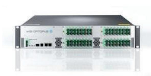
LX 37 is an optical amplifier based on YEDFA technology for use in HFC and FTTx networks. The system is available with different output power and various numbers of outputs. The W-Type with integrated WDM filters for PON networks is specifically developed for RF Overlay networks.
