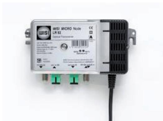
The LR 92 is an extremely low-noise optical receiver. Because of the high output level it is particularly well suited for direct house distribution. The measurement point can be displayed through the LED and the DC, in the range of -8 to +1 dBm. The return path transmission is ensured through the 1310 nm Fabry-Perot laser. Its compact design requires a minimum amount of space, and the built-in measuring socket allows control of the signals.
