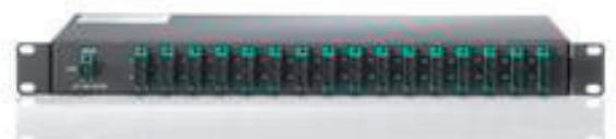
The LP 90 W 0132 is an optical PLC splitter with included WDM filter. It is equipped with one CATV input, 32 IP inputs and 32 COM output ports. Its wavelength is in the range 1540...1620 nm for the CATV downstream signal and 1260...1500 nm for the IP signal.
