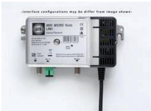
The LR 91 W is a compact receiver for CATV distribution networks and RF overlay. The integrated WDM filter makes it possible to decouple the xPON wavelengths in addition to the CATV. It has a high output level up to 100 dB $\mu$ V in the frequency range up to 1 GHz.
