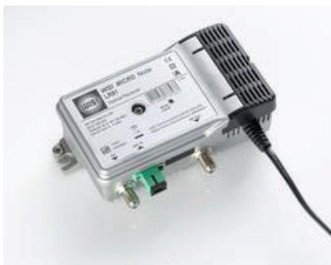
The LR 91 is an extremely low-noise optical receiver. Because of the high output level it is particularly well suited for direct house distribution. The measurement point can be displayed through the LED and the DC, in the range of -8 to +1 dBm. Its compact design requires a minimum amount of space, and the built-in measuring socket allows control of the signals.
