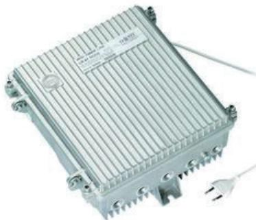
Optical node with integrated fibre management. Plugin modules for return path transmitter, diplex filter and splitter/taps. Local configuration with OH 41 handset or Android app via Bluetooth. Remote management via HMS or DOCSIS 2.0 transponder.
