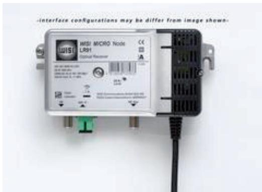
The LR91 W 1550 is a compact receiver for CATV distribution networks and RF overlay. The integrated, very narrow-band, WDM filter allows the out-coupling of the xPON wavelengths, which are additionally connected to the CATV. It has a high output level up to 100 dB $\mu$ V in the frequency range up to 1 GHz.
