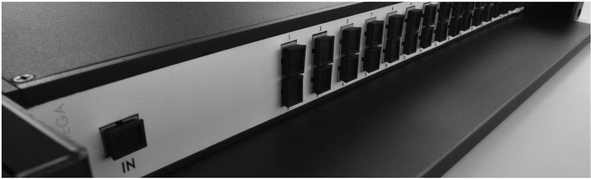
*ftth splitter, 19-inch rack type with 32x wdm module*
